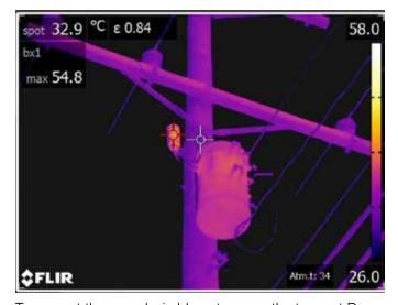
To prevent these undesirable outcomes, the team at Davey offers infrared inspection services that can detect, measure and monitor the heat emitting from utility equipment. Heat sensed by infrared technology can be precisely measured and quantified, helping to identify equipment that has
